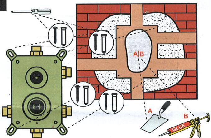
FIXOVANÍ BOXU • FIXOVANIE BOXU • FIXING OF BOX • MOCOWANIE BOXU • FIXAREA CASETEI
